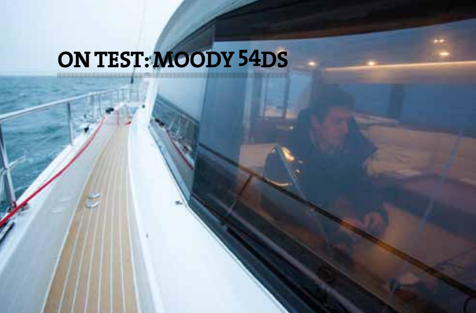
▲ Side decks Bulwarks are high to give a feeling of security when walking round the deck. Stanchions are carefully curved to allow genoa tracks to be mounted here
