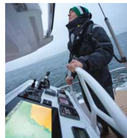
▲ Bus system Moody chose to install a C-zone digital switching bus system as standard, which reduces cable runs and provides intuitive systems monitoring on touchscreen displays. But, perhaps aware that some owners will not want to rely on such a modern system offshore, Moody has commendably also installed a back-up 12V system so that the main powered sailing and navigation systems can still be operated independently of the bus system
