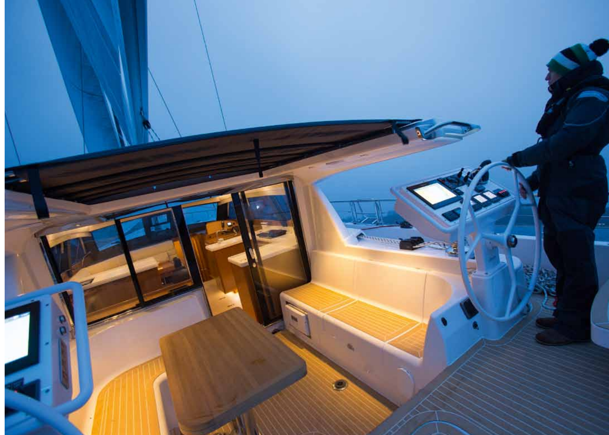
▲ Bus system Moody chose to install a C-zone digital switching bus system as standard, which reduces cable runs and provides intuitive systems monitoring on touchscreen displays. But, perhaps aware that some owners will not want to rely on such a modern system offshore, Moody has commendably also installed a back-up 12V system so that the main powered sailing and navigation systems can still be operated independently of the bus system
