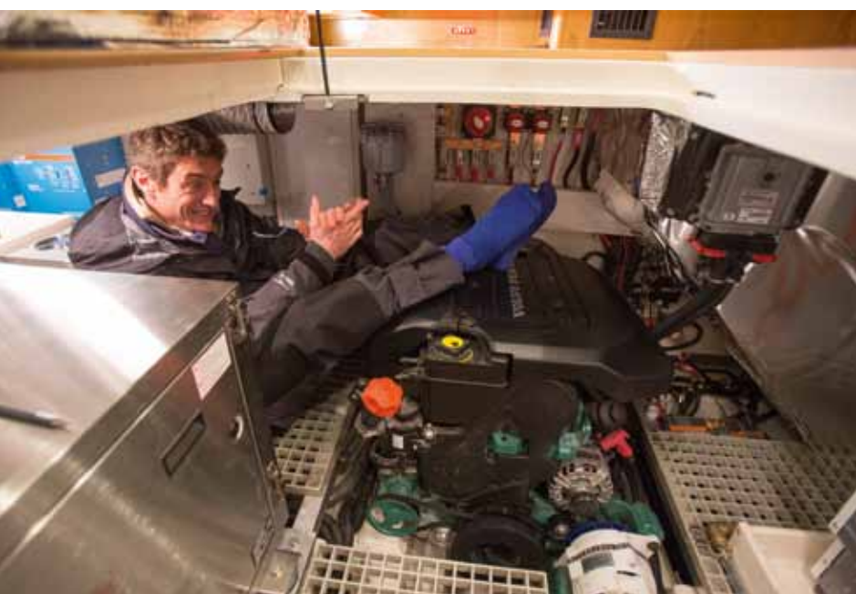
▲ Engine room Thawing out – the soleboards of the decksaloon lift to reveal a prize asset of the 54DS, a spacious and impressively installed engine and machinery room. There is space enough to provide all-round access to the engine and genset, plus chargers, fuses, aircon units, etc. A washing machine can also be installed here, accessed through the day heads
